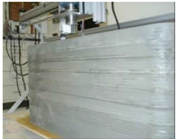
A robot builds one of the first walls ever constructed entirely by automated processes in the University of Southern California lab of Professor Behrokh Khoshnevis, February 2004.
