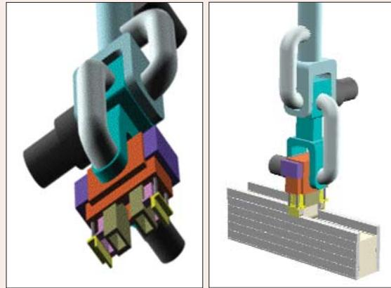
For example, plaster as the outer surface material and concrete as the core structural material may be co-extruded by the CC nozzle.
